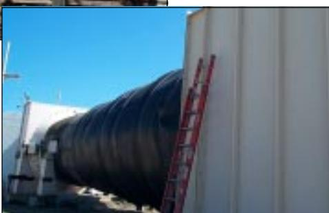
Underground mines use special air systems to channel fresh air through the mines. Large fans pull fresh air down the **intake air shaft**.
